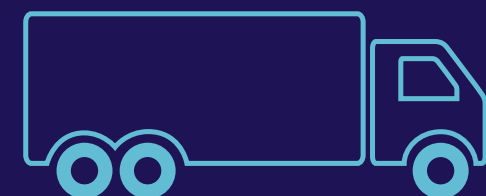
Torton truck 3 axles 10 wheels 15 tons
